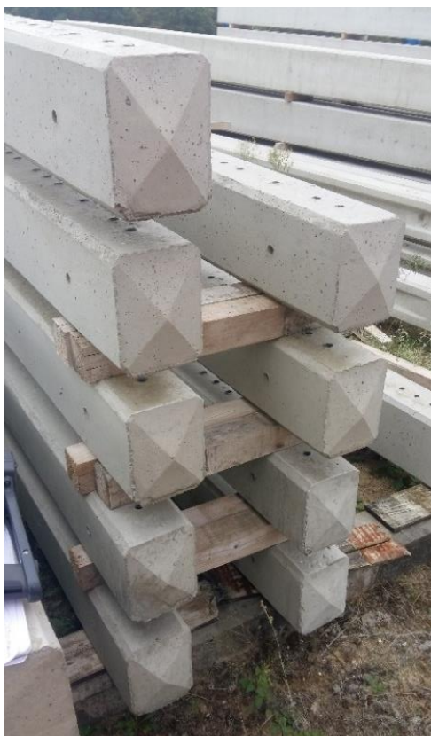
Figure 27 – Têtes de poteaux
