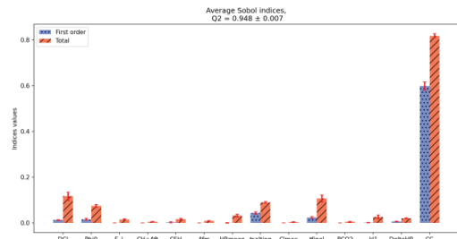
Fig. 3. Average values of the first and total order indices for the surrogate model computed.
